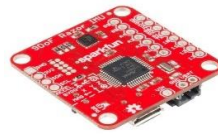
Figure 9. SparkFun 9DoF Razor IMU (size: 3cm by 3cm)
