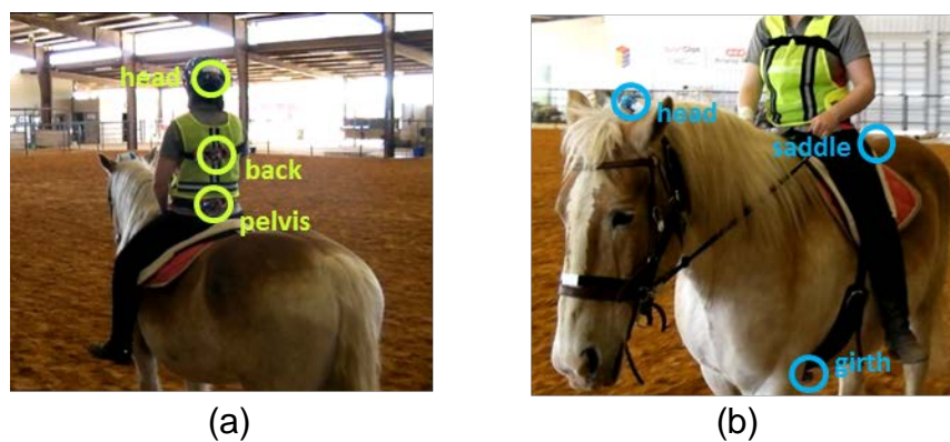
Figure 3. Wearable sensor locations for (a) the rider and (b) the horse.
